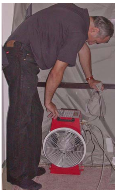
Figure 3.17 and 3.18 Testing the airtightness of a wall during the construction stage (left) in order to verify airtightness. Air leaks are traced e.g. with smoke and anemometer measurements (right)
