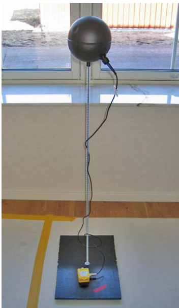
Figure 3.9 Measuring the operative temperature in an apartment in a passive house in Frillesås, Sweden.
