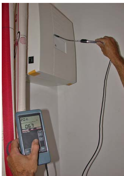
Figure 3.17 and 3.18 Testing the airtightness of a wall during the construction stage (left) in order to verify airtightness. Air leaks are traced e.g. with smoke and anemometer measurements (right)
