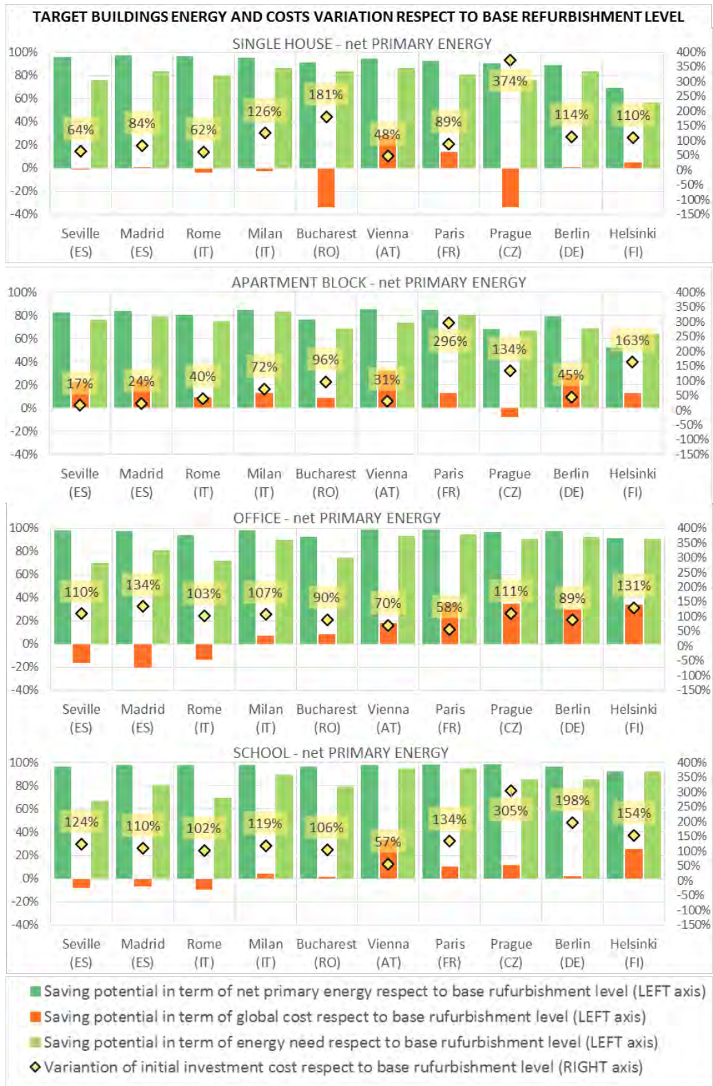
Figure 24. Target buildings energy and costs variations respect to base refurbishment level (graphs and tables) - min. net primary energy (nZEB) selections
