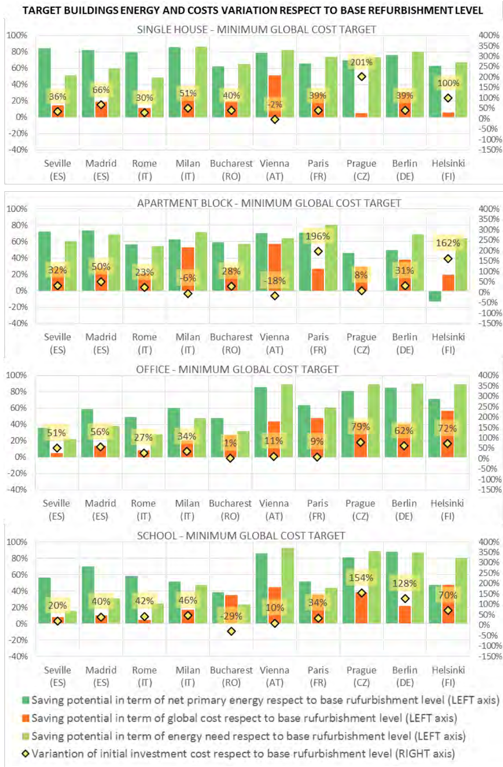
Figure 25. Target buildings energy and costs variations respect to base refurbishment level (graphs and tables) - min. global cost (cost-optimal) selection
