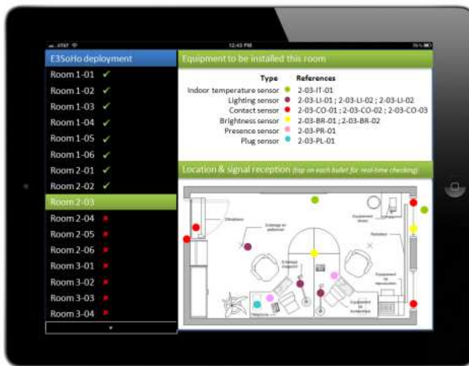
Figure 43: Possible user interface for a tablet-based application supporting the installation and deployment of ICT sensors and meters within a building
