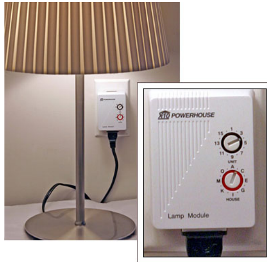
Figure 7. A complete X10 lamp control module.
