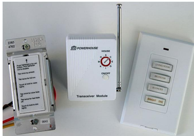
Figure 6. some most common hard-wired and wireless X10 products.
