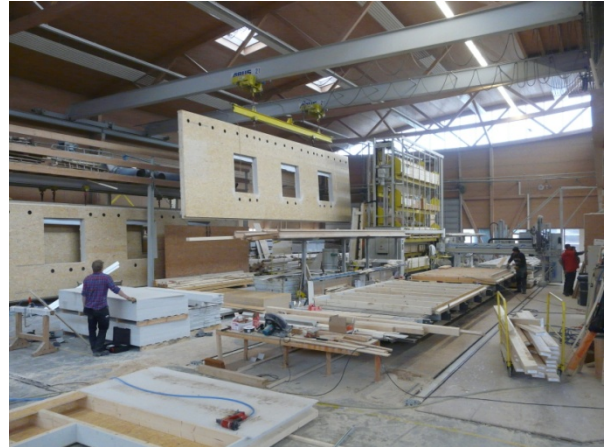
Figure 12 - Production line of timber frame elements
