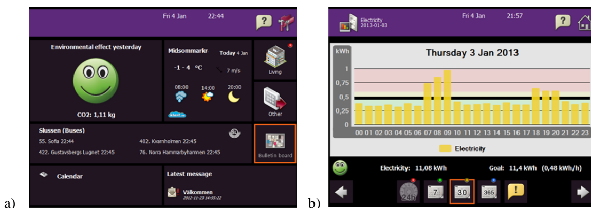
Figure 7: a) MANODO Energy display showing environmental load as well as a number of other service functions. b) Bar chart showing the hourly energy use. (MANODO, 2014)
